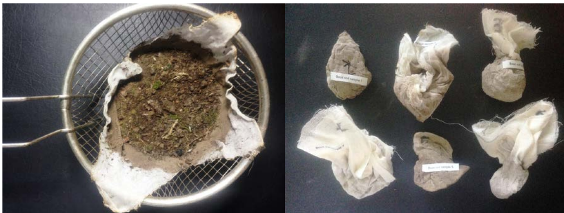
Filtering soil & detritus through muslin and sieve
